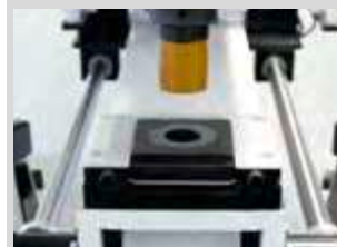
Die bed holder. Tool changes can also be carried out when control cabinet door is fitted
