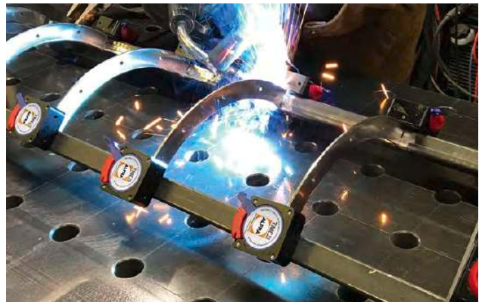
Instead of complicated clamping: The TMC 70 for easy fixing of metal parts for welding work
