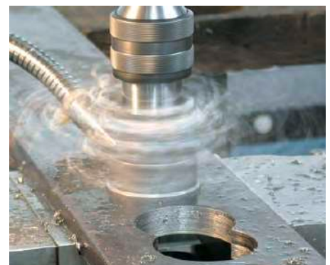
Drilling in flat steel
