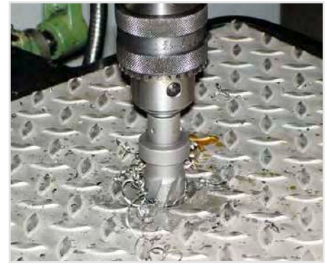
Drilling structured sheet metals
