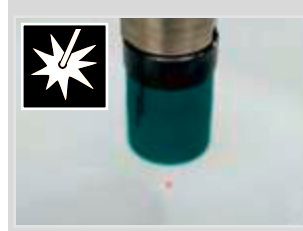
Laser pointer for optical display of tool centre and power bank
