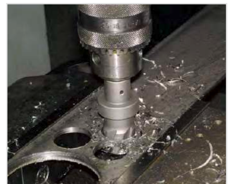
Drilling flat steels
