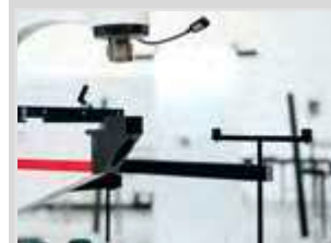
Pivoting support arms, height adjustable, each with 3 rubber supports
