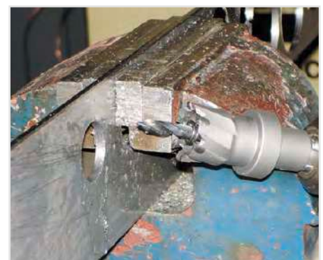
Free-hand drilling up to Ø 30 mm
