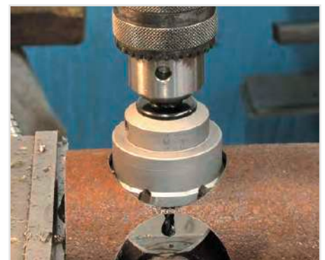
Drilling in pipes
